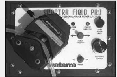
When the pump is switched on, the red indicator will light. Select the flow direction desired. Note that the middle station on the switch is the "off" position. When changing pump direction, turning the unit off for a minute will extend the life of the motor. The speed control knob can adjust the flow rate from 50-1900 ml/min. Once the flow rate is set, the Field-Pro will maintain this flow rate.
