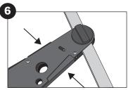
6) Squeeze the Grip to line up the holes in the Grip with the holes in the Body. Bend the extra 4 top 5 feet of tubing above the tubing clamp around and fit it through the Body Tubing Holder. Release the Grip. The discharge end of the tubing will then be held in place.
