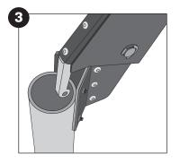
3) Fasten the WLP-100 Lever Pump on the top edge of the well casing or surface protective casing.
