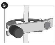
5) Fit the tubing in the appropriate cutout in the Tubing Clamp, with 4 to 5 feet of tubing protruding above the clamp. Close and tighten the tubing clamp with Knob 2, located at the tubing clamp.
