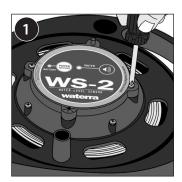
The batteries can be accessed by removing the two screws located on the Front Panel above and below the label. Remove these screws with a Phillips screwdriver and then carefully lift the Front Panel from the front hub. Turn the Front Panel upside down and place the two screws in the panel.
