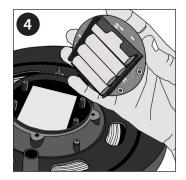
Once the Main Circuit Board is removed, turn it over and replace the worn AA cells with four fresh Duracell AA batteries. Be sure to orient the batteries in accordance with the directions supplied on the battery pack. Return the Main Circuit Board to the reel by carefully lining up the pins with the connectors (4 pin connector on the left, 6 pin connector on the right) and press the Main Circuit Board into position.
